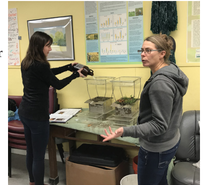
University of Vermont Extension Service soil specialists use a rainfall simulator to demonstrate the effects of cover crops on runoff and infiltration.
